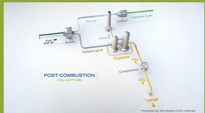
**Post-combustion** processes separate CO2 from combustion exhaust gases. CO2 can be captured using a liquid solvent or other separation methods. In an absorption-based approach, once absorbed by the solvent, the CO2 is released by heating to form a high purity CO2 stream.
